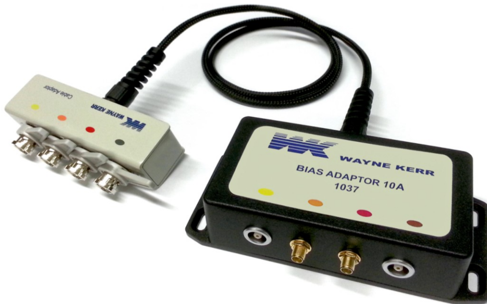
Fig. 1 1037 showing connection outlets to test head.
