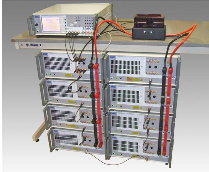
1036 Fixture in a 200A dc bias current system (8 x 3265B)
